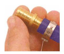
4. Position the open jaws of the PinchLok Tool over the tabs of the Clamp and squeeze. The ratchet effect of the PinchLok Tool will not allow for an improper connection. The PinchLok Tool will release automatically when the connection is complete.
